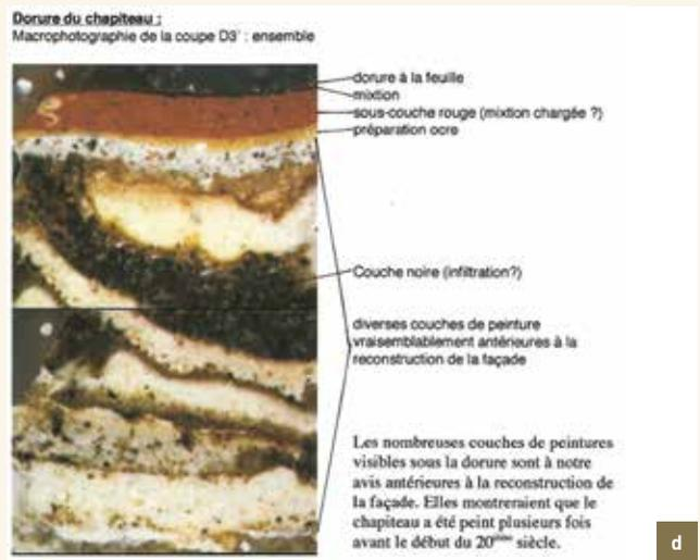
*L'Âne/Den Ezel*. a) View of a capital with stratigraphic sampling (© M. Decroly, 2002); b) Detail of stratigraphic sampling D2. 1. Stone. 2. Black layer (sealer or black crust). 3. Ochre mix. 4. Red undercoat. 5. Gilding on mixtion (© M. Decroly, 2002). c) View of the volute of a capital with sampling D3 (© M. Decroly, 2002); d) Macro photograph to see different layers of paint, suggesting that the capital has been recovered (© KIK-IRPA, 2002).
